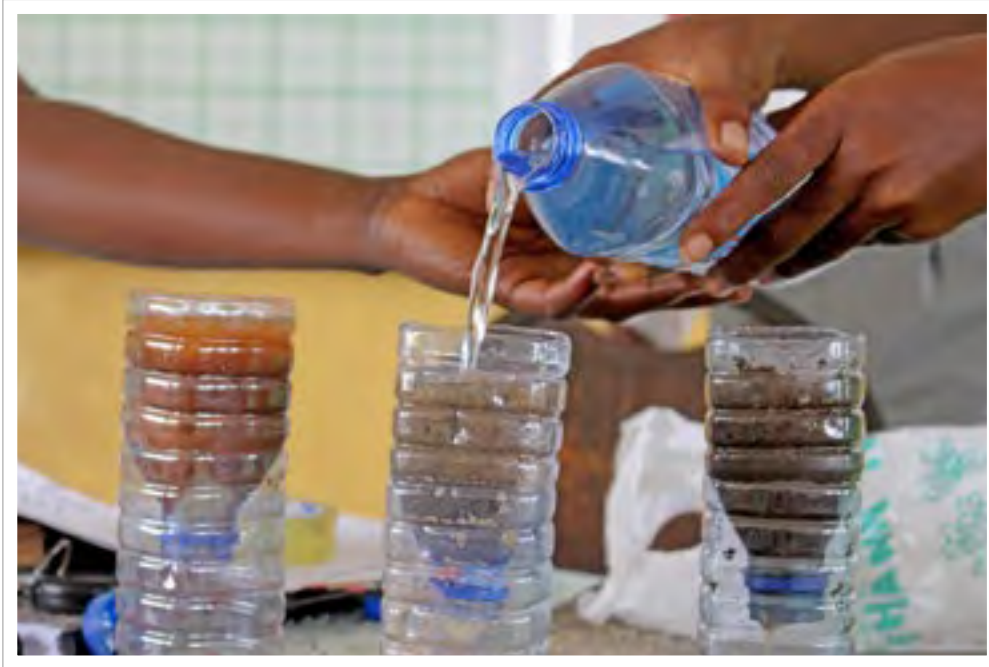
Figure 102. Testing water retention
